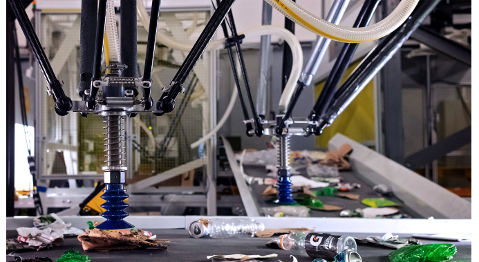
Figure 1. Example of parallel robots in action in the waste sorting machine from AMP robotics (I x 4 Omron robot equipped with the P30 rigid platform) [8].
