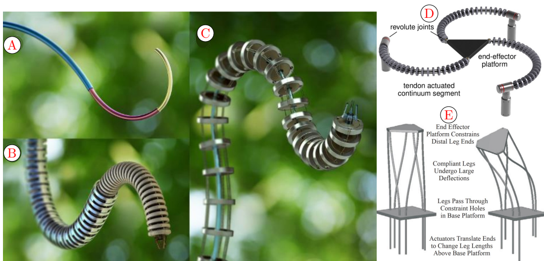
Figure 1.1: Examples of different types of continuum robots in the literature A) Concentric tube robot (CTR) actuated by axial rotation and translation of pre-curved tubes (image from [Chikhaoui 18a], online ), B) Hybrid continuum robot with a combination of tendon-driven segments in a concentric assembly manner [Chikhaoui 18a], C) Tendon-driven continuum robot with extensible segments, using self-repelling magnetic spacer disks, (image from [Chikhaoui 18a], online ), D) Planar tendon actuated parallel continuum robot [Sven 21], E) Stewart type compliant legs parallel continuum robots [Bryson 14]
